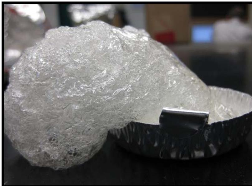
Figure 39: Foamed MF sample with a catalyst loading level of 0.28 wt% at 140°C
