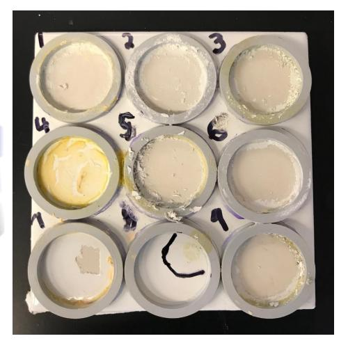
The only paint stripper that demonstrated performance similar to the methylene chloride-based paint strippers and did not contain other Benchmark 1 chemicals (such as toluene, methanol, and naphthalene) was the Super Remover Professional Grade product.
