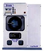
Inner-Tite chose to replace its degreasing equipment with a new technology adapted from the dry cleaning industry (see left). Manufactured by Forenta, the unit's design and operation are similar to that of a washing machine. Workers load bins of parts into the wash bay, then close and seal the door. The 13-minute cleaning cycle is entirely automated and a sensor prevents the wash bay door from being opened again until the drying period is completed.
