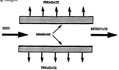
Figure 1. Schematic Representation of Crossflow Filtration
