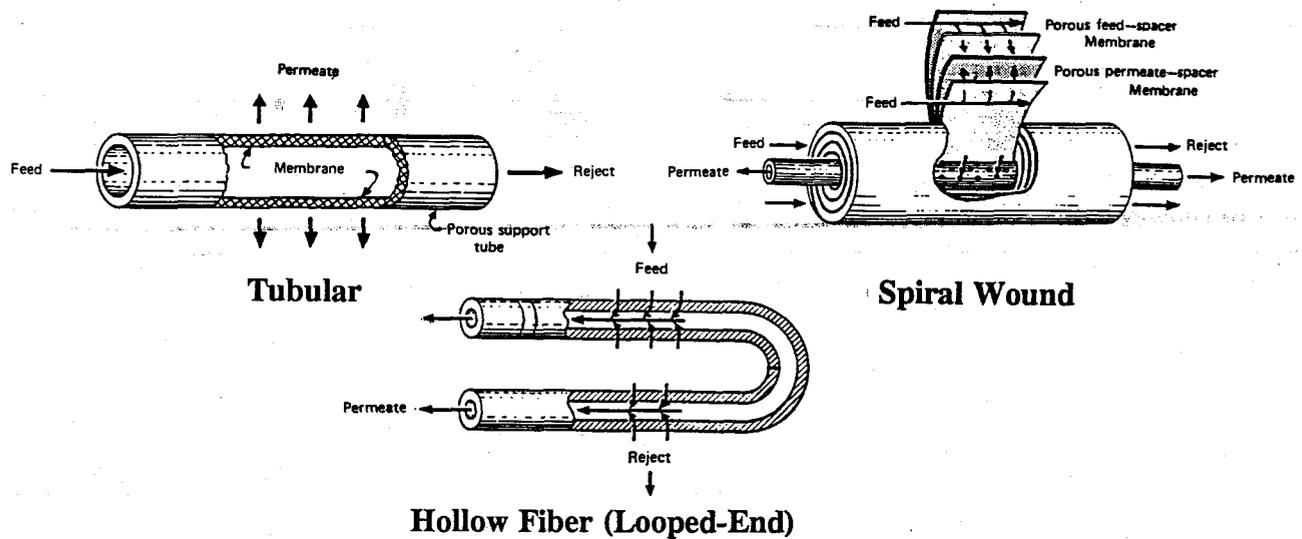
Figure 2. Membrane Configurations Used in Closed Loop Cleaning Membrane Modules<sup>2</sup>
