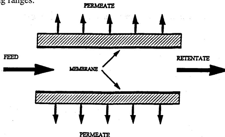
Figure 1. Schematic Representation of Crossflow Filtration
