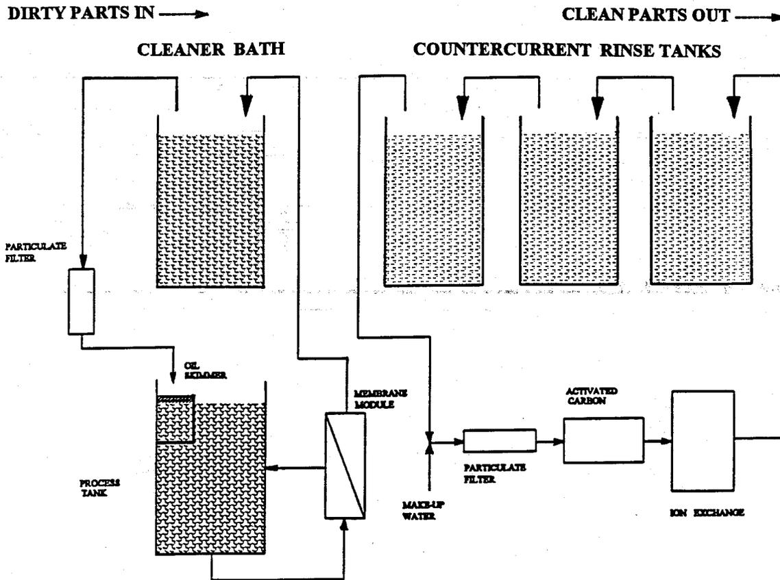
Figure 3. Simplified Closed Loop Aqueous Cleaning System
