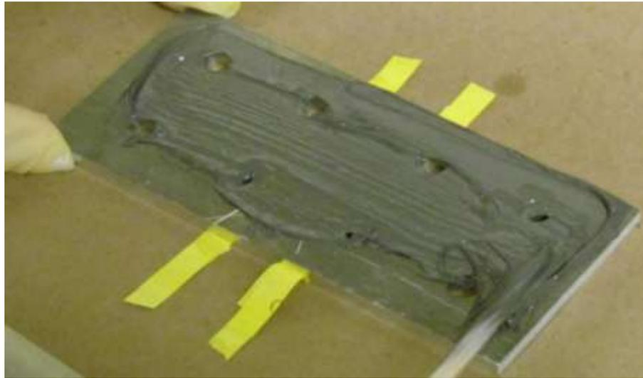
FIGURE 4.6.2 APPLICATION OF SEALANT ON TOP SIDE OF BASE PLATE
