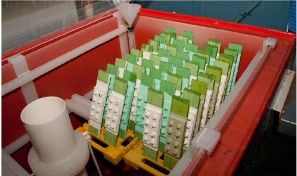
FIGURE 5.2.2.1 TEST VEHICLE ORIENTATION FOR FIRST 168 HRS OF EXPOSURE TO SO<sub>2</sub> SALT FOG
