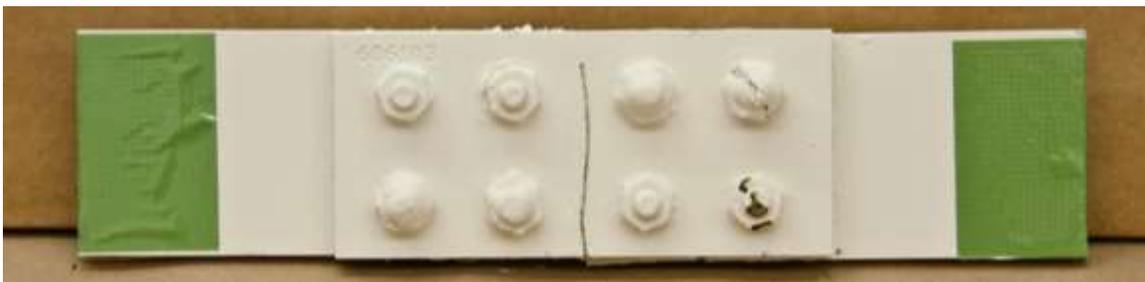
FIGURE 5.2.1.3 TEST VEHICLE WITH THE ENDS TAPED BEFORE EXPOSURE TO SO<sub>2</sub> SALT FOG
