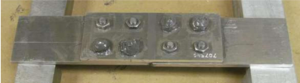
FIGURE 4.6.9 SEALANT APPLIED TO CORRESPONDING NUTS OF FASTENERS. STRIP OF SEALANT APPLIED TO SURFACE IN BETWEEN
