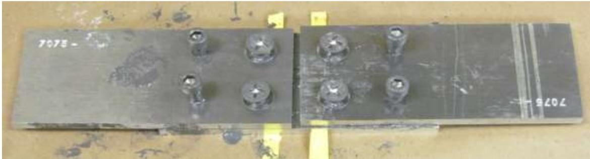
FIGURE 4.6.6 FASTENERS INSERTED INTO FRESHLY MATED PANELS
