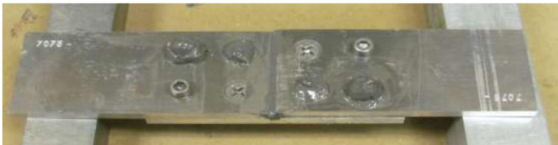
FIGURE 4.6.8 SEALANT APPLIED OVER FASTENER HEADS
