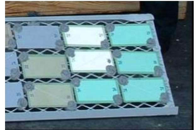
Primers with rare earth inhibitors during a six month field evaluation on the John C. Stennis
