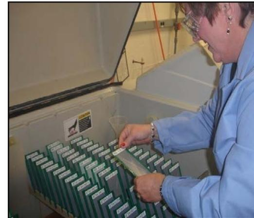
**Technician loading test panels
