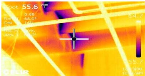
*This Image shows the conductive heat loss of the concrete roof T's on the interior side of the roof overhang. Planned future renovations of the exterior façade will eliminate a potential dew point concern on very cold winter days*
