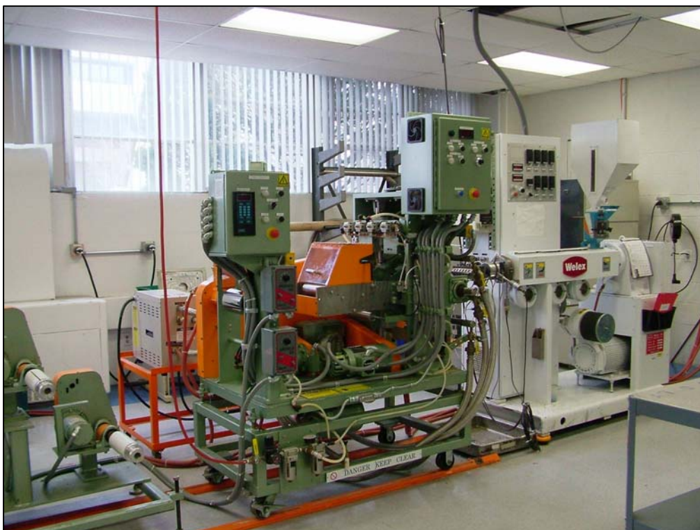
Figure 6 – Equipment used for sheet extrusion (Welex single-screw sheet extruder).
