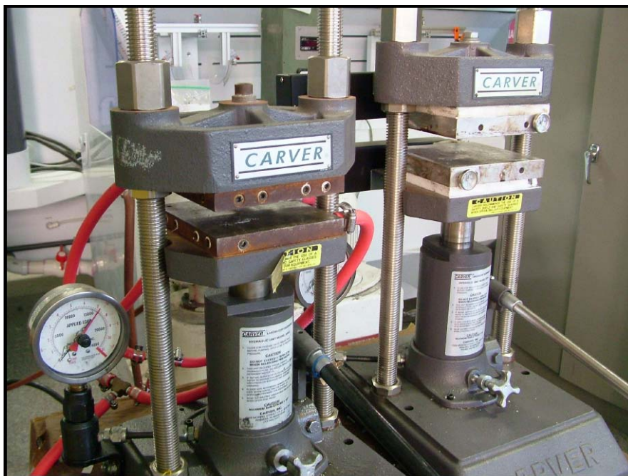
Figure 7 – Equipment used for compression molding (Carver press).
