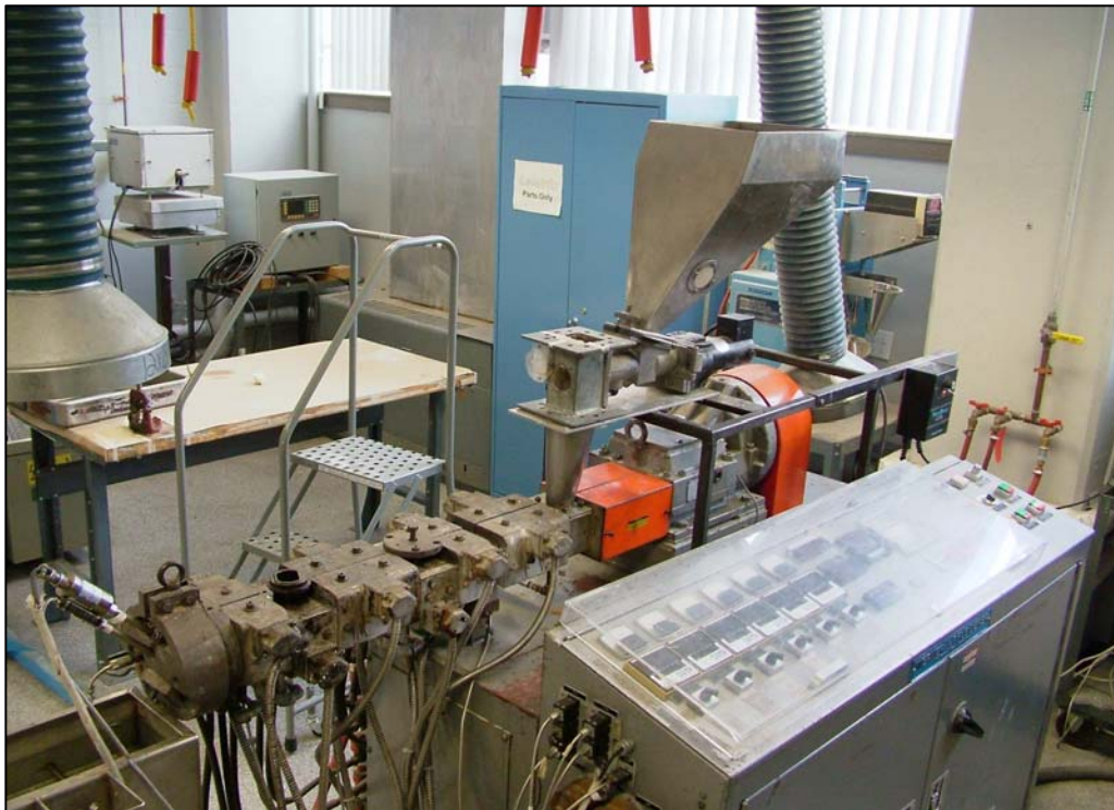
Figure 5 – Equipment used for melt compounding (Werner & Pfliederer ZSK-30 twin-screw extruder).
