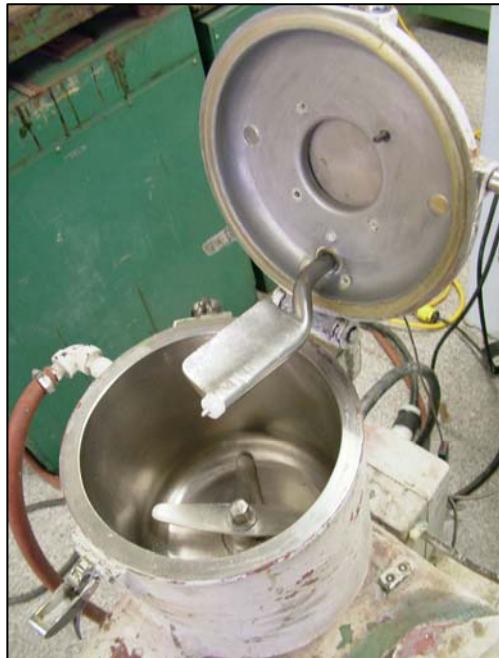
Figure 4 – Equipment used for dry-blending (Henschel high-intensity mixer).
