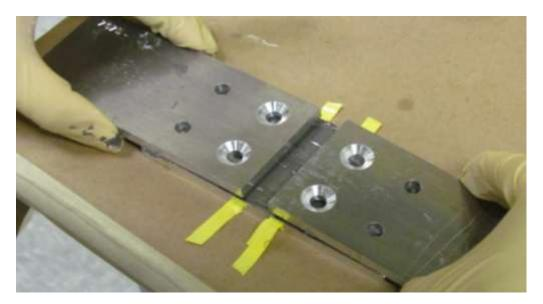
FIGURE 4.6.4 MATING OF TOP PLATES TO BOTTOM PLATE
