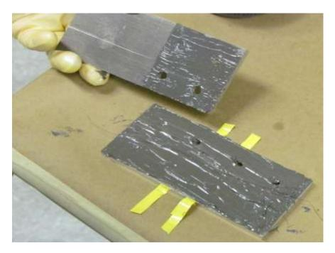
FIGURE 4.6.3 APPLICATION OF SEALANT ON BOTTOM SIDE OF TOP PLATES AND ADDITION OF TWO WIRES TO TOP SIDE OF BOTTOM PLATE
