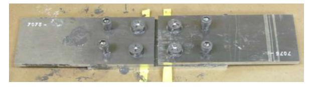
FIGURE 4.6.6 FASTENERS INSERTED INTO FRESHLY MATED PANELS
