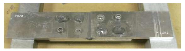
FIGURE 4.6.8 SEALANT APPLIED OVER FASTENER HEADS
