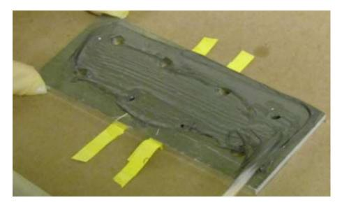
FIGURE 4.6.2 APPLICATION OF SEALANT ON TOP SIDE OF BASE PLATE
