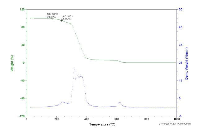
Figure 2: TGA data from crude CBDO-DGE (1<sup>st</sup> synthesis) following crosslinking with TETA.
