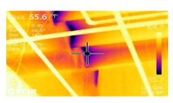
This Image shows the conductive heat loss of the concrete roof T's on the interior side of the roof overhang. Planned future renovations of the exterior façade will eliminate a potential dew point concern on very cold winter days
