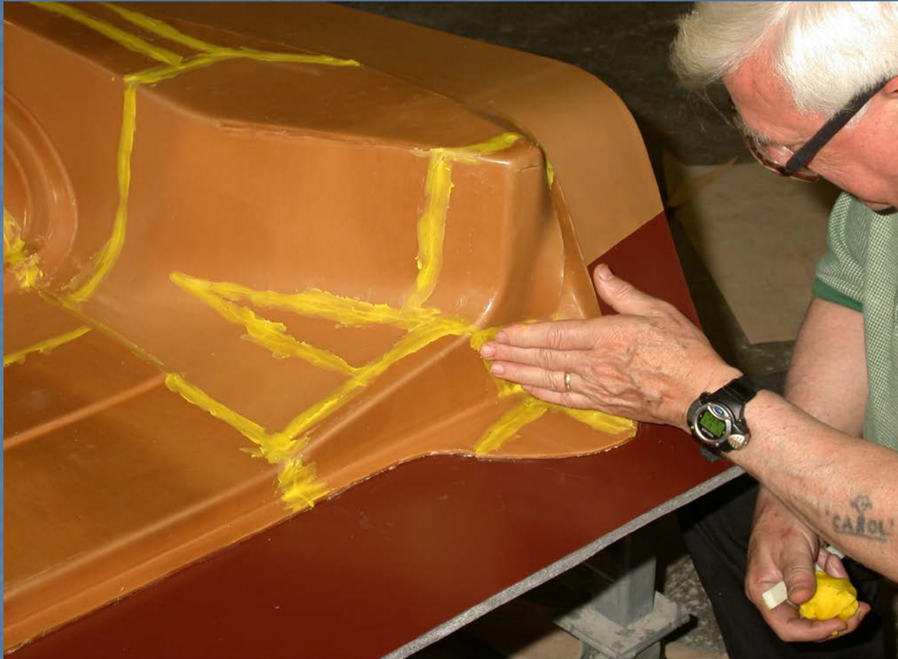
Application of filler material to fill gaps and smooth surface
