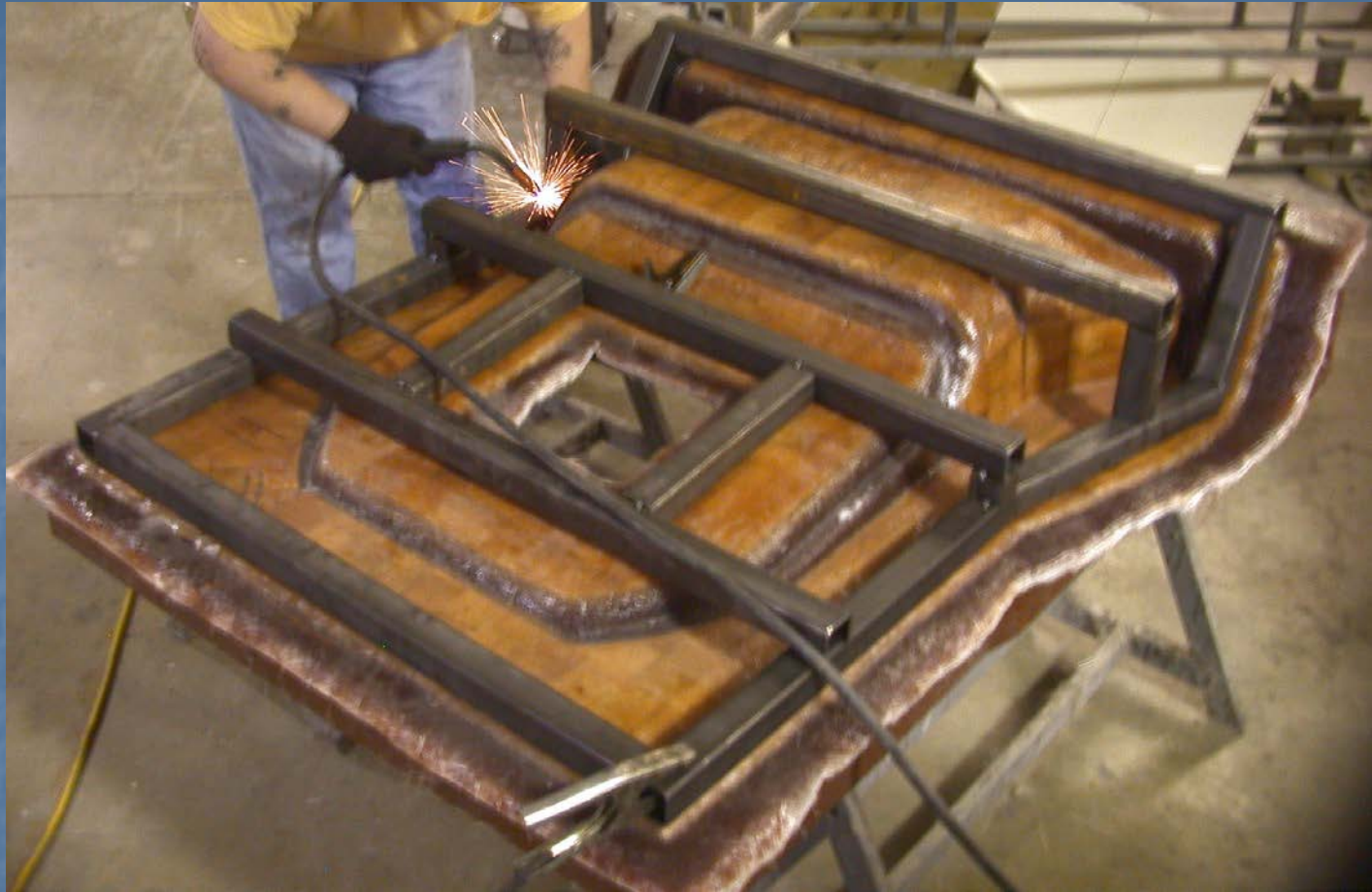
Back of female tool mold Adding reinforcement to give the mold strength
