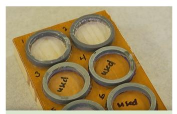
Test board used to demonstrate the effectiveness of the alternative paint stripper at the TURI Laboratory
