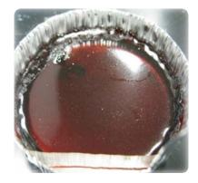
Figure 18: ELO - PEI cured at 160°C for 18 hrs
