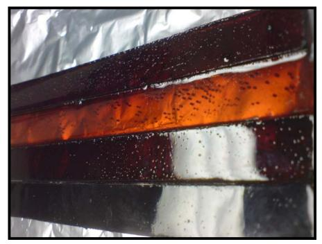
Figure 42: Flexure bars with bubbles made of ELO - PEI (1:1.4) cured at 160°C for 18 hrs without and with Cloisite 30 B (nanoclay) loading level of 2 %wt.
