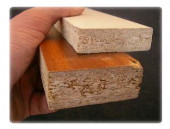
Figure 1: Particleboard coupon
