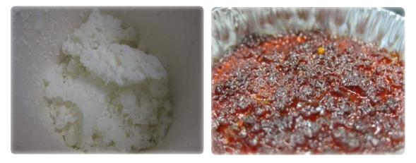
Figure 35: Chunks of L-lysine (left) and cured sample of L-lysine and ELO (right)
