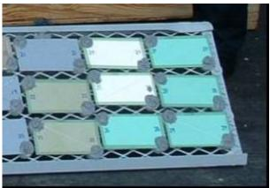
Primers with rare earth inhibitors during a six month field evaluation on the John C. Stennis
