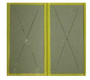
Chromate primer on CrCC after 3000 hours in ASTM B117 salt spray testing
