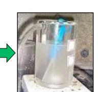
Alkaline Degreasing 5 min at 55°C
