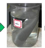
Acid Activation 1 wt% H<sub>2</sub>SO<sub>4</sub> 5 min at 50°C
