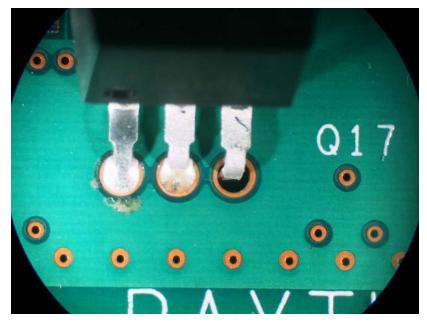
TO220, Insufficient solder, Test vehicle 22, Q17
