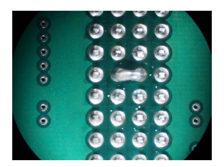
200 pin connector, Solder bridge, Test vehicle 28, J5
