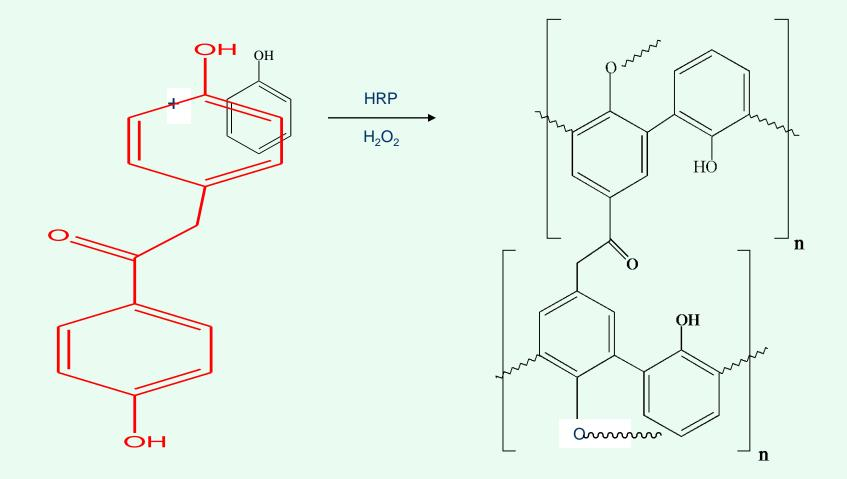
Phenol was used as a spacer with the BHDB units to increase solubility of the reaction mixture
