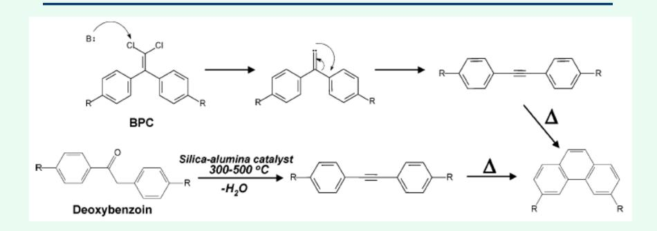
Investigations into decomposition pathways of BPC-containing polymers suggest that char formation may proceed through diphenylacetylene derivatives
