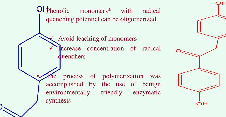
MHDB - 4-methoxy4'-hydroxydeoxybenzoin
