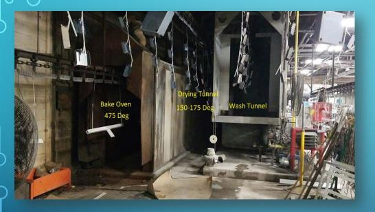
Both bake oven and drying tunnel have their own burners. Both exhaust directly outside.
