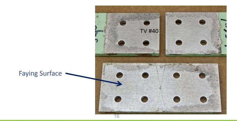
Corrosion analysis after exposure in salt fog chamber.
