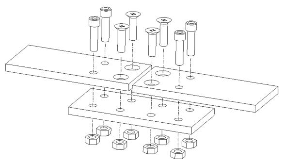
8 stainless steel fasteners (4 with 100 degree countersunk heads, and 4 with socket heads)
