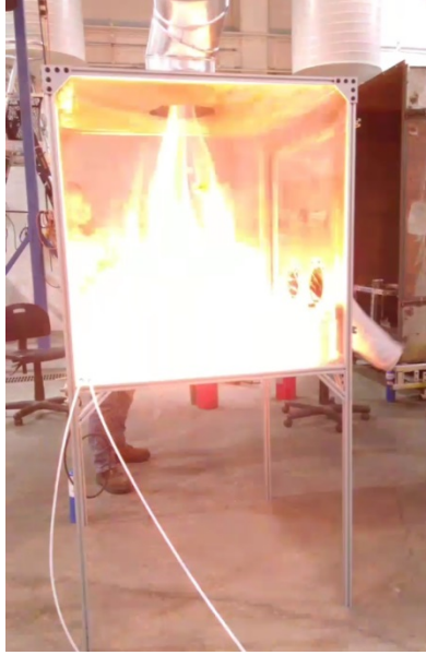
Figure 5: Combustion event inside the glove box
