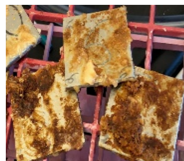
Macaroni and cheese placed on stainless steel coupons, heated to 180°F for 3 hours
