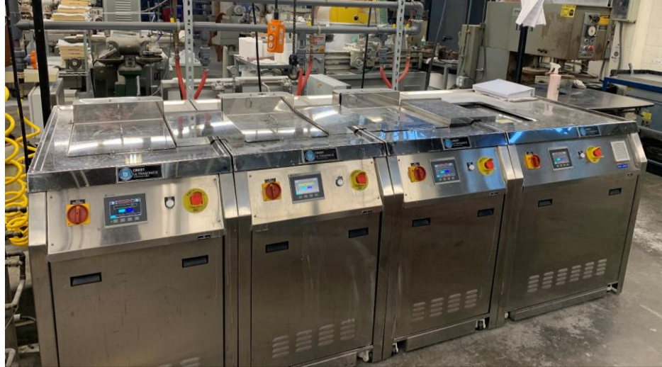
New Crest Ultrasonics vapor degreaser
