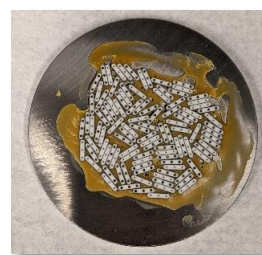
Dirty parts with brown wax residue
