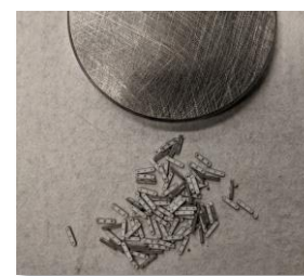
Clean parts after brown wax removed
