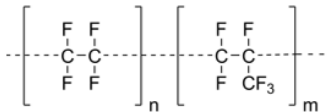
FEP Fluorinated ethylene propylene polymer [25067-11-2] polymer with repeating units that include 3 contiguous perfluorinated carbons
