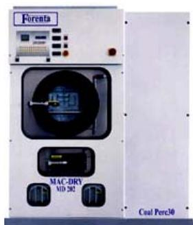
Inner-Tite chose to replace its degreasing equipment with a new technology adapted from the dry cleaning industry (see left). Manufactured by Forenta, the unit's design and operation are similar to that of a washing machine. Workers load bins of parts into the wash bay, then close and seal the door. The 13-minute cleaning cycle is entirely automated and a sensor prevents the wash bay door from being opened again until the drying period is completed.
