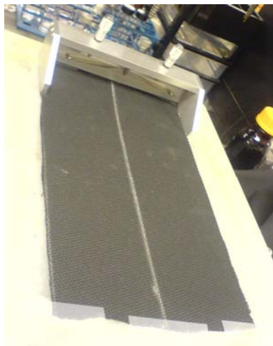
Figure 15. Blade knife coating of automotive textile
