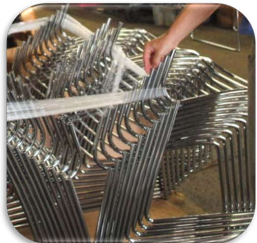
Typical product with nickel trivalent chromium plating
