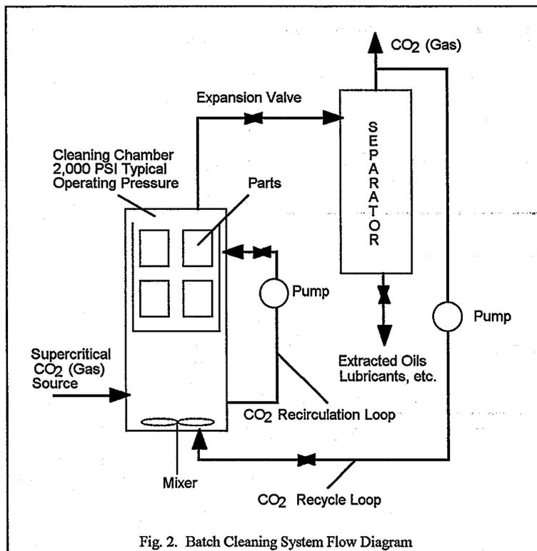
Fig. 2. Batch Cleaning System Flow Diagram
