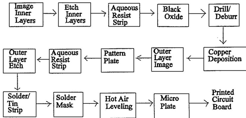
Fig.1. Printed Circuit Board Flow Diagram.
