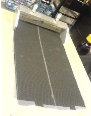
Figure 15. Blade knife coating of automotive textile
