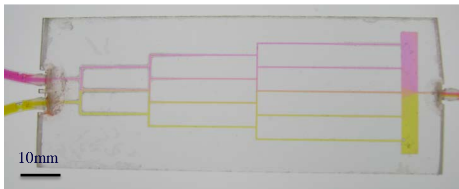
Fig 6. Fluorescein- (left) and rhodamine-dyed (right) water inputs flow at 0.05 mL/min and diffusively mix.
