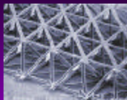
Trusses, 1-100 μm MEM, Pure Nickel
