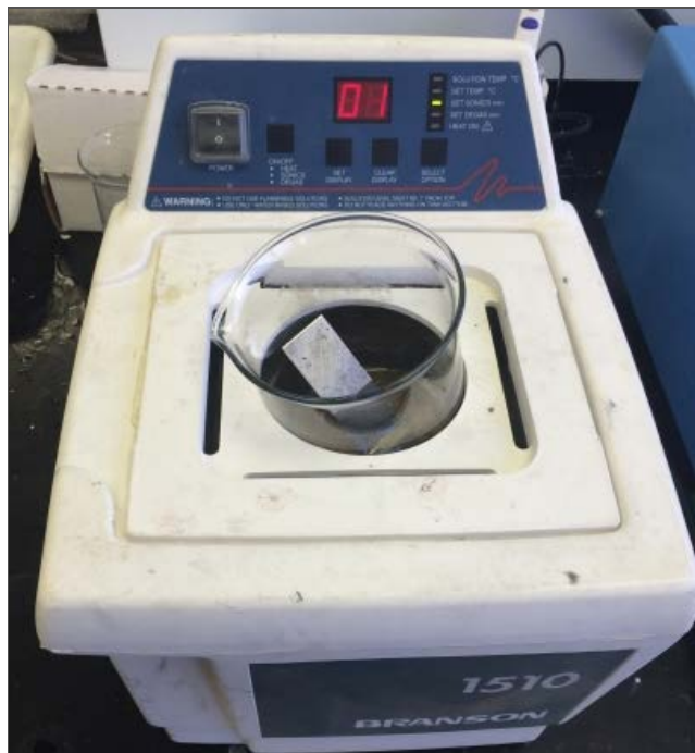
Figure 6: Sealant removal ultrasonic bath test
