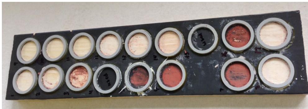
Figure 8: Wood Panel with Ring Gaskets After Testing
