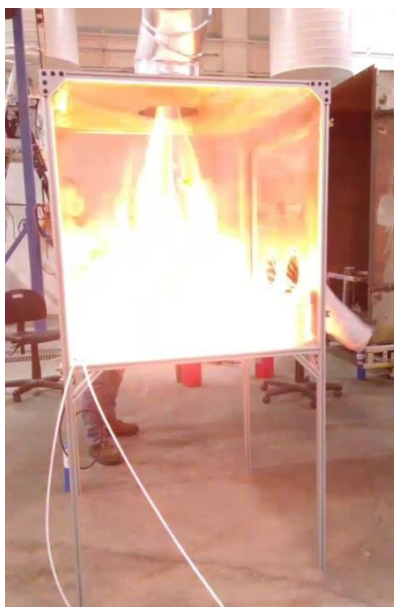
Figure 6: Combustion Event Inside the Glove Box
