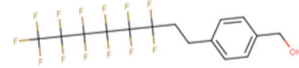
4-((Perfluorohexyl)ethyl)phenylmethanol [356055-76-0] six perfluorinated carbon alkyl chain with benzene ring as functional group
