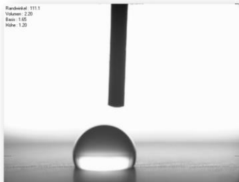
Big contact angle low surface energy
