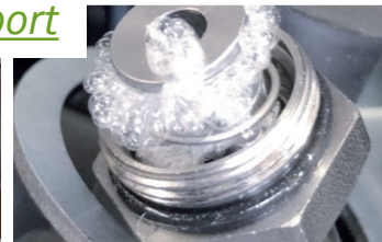
Figure 1: Polymerized refrigerant in connecting piece
